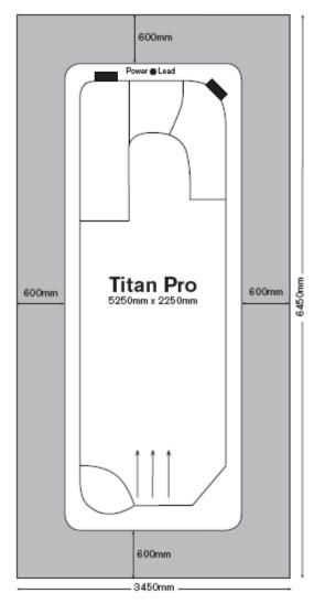
In Decking: If you are sinking your pool and decking around it please remember to build the decking to allow access to the electrical compartment and all components. Please ensure the electrical compartment has some ventilation for correct functioning. If decking up to/around pool, we would recommend decking after installation.
