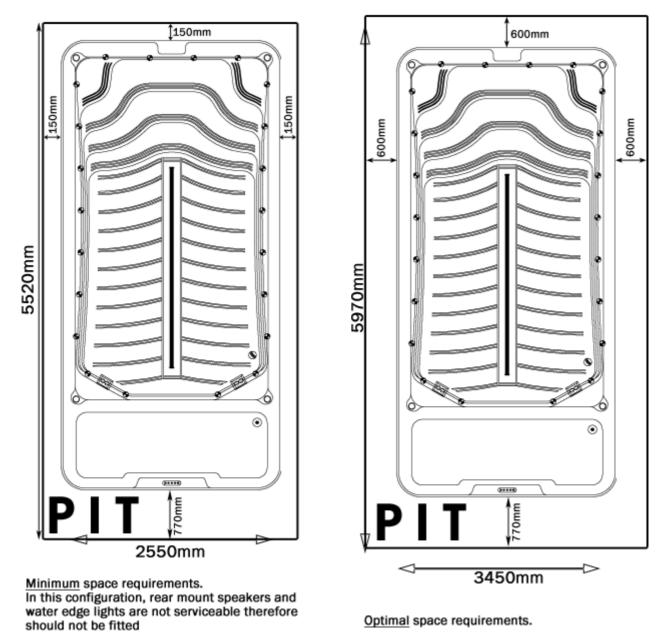
For **minimum** pit size, please allow 150mm gap on all four sides of your pool, with a further 170mm extension (770mm total) at the inspection pit end where the components will need to be accessed. In a pit of this size, rear mounted speakers and water edge lights will not be serviceable and therefore cannot be installed.
