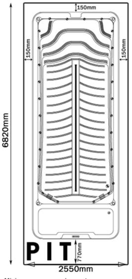
Minimum space requirements. In this configuration, rear mount speakers and water edge lights are not serviceable therefore should not be fitted
